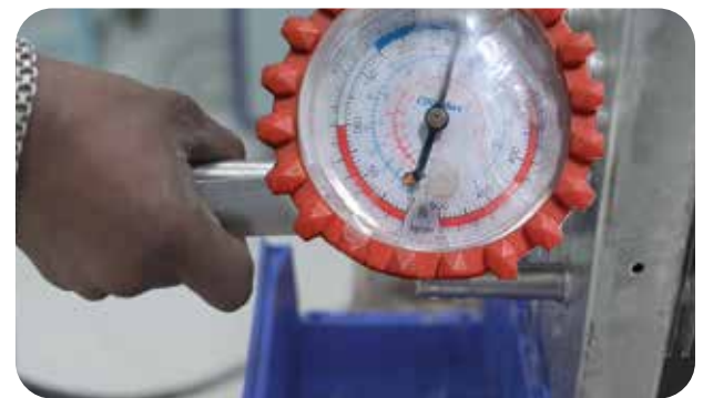
Individual Tube Pressure Test
